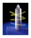
Vinotrak is especially designed to remove microorganisms. Vinotrak filter element is manufactured with an innovative filter media made of polypropylene nanofiber with dimensions that varies from 0,5 to 0,8 micron supported by a borosilicate microfiber.
